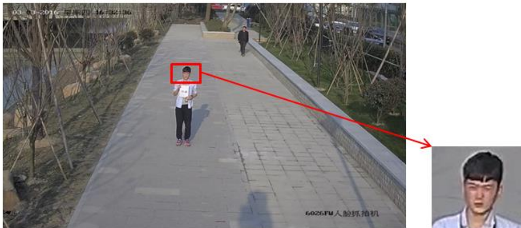
The scenario is too large and the face recognition rate is low
